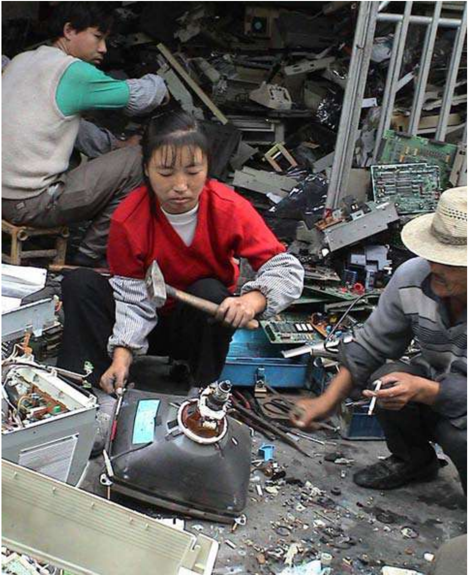
Electronic waste dismantling of monitor to remove copper yoke, Guangdong, China, 2002. (Photograph courtesy of Basel Action Network.)
