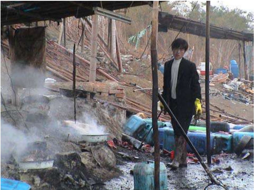
Dismantling electronic waste and removing gold from circuit boards with aqua regia, Guiyu, China, 2002. (Photograph courtesy of Basel Action Network.)
